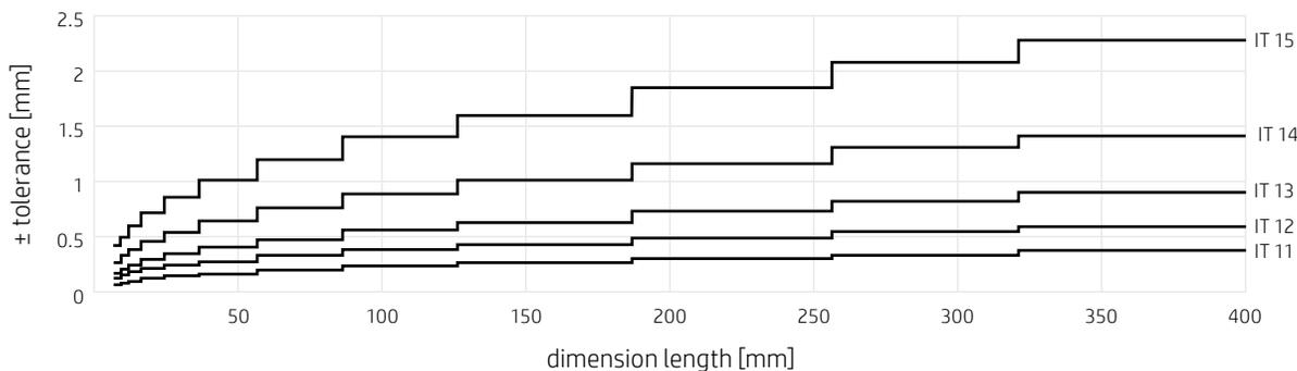
Figure 8. Tolerance range vs. dimension length
