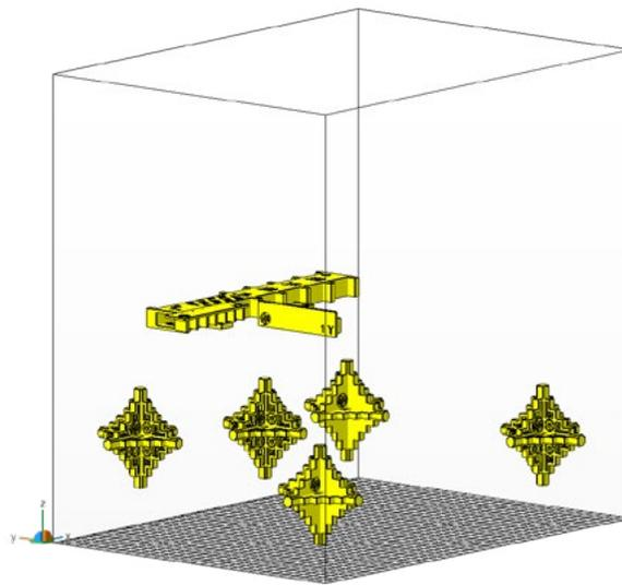
Figure 2. Dimensional test parts in half bucket part property test build. Mechanical and look and feel parts are hidden to highlight location of dimensional parts.
