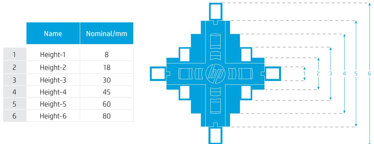
Figure 3. Dimensional fiducial nominal dimensions of the snow star part
